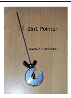
Pointers are a handy device that you can attach to a safe lock and allow the user to plot your way though a lock that you are picking.
