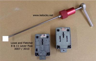
This is <u>one</u> pick that comes with a removable tip that can be changed for pin or pipe.
