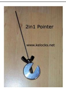
Pointers are a handy device that you can attach to a safe lock and allow the user to plot your way though a lock that you are picking.
